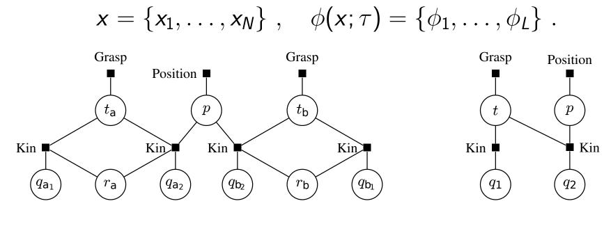
q robot joint configuration *t* transformation object-gripper r mobile base pose *p* position of the object
